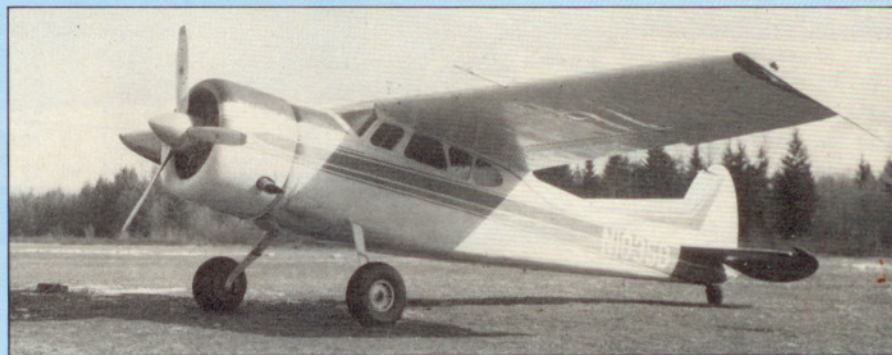
More than half of the 190/195s built still are around. Most have been modified, as the one above, and look entirely different from the prototype. Changes include flatter, more powerful engines, such as the 450-hp Pratt & Whitney Wasp Jr., "booster" wingtips, larger wheels and a dorsal fin.
