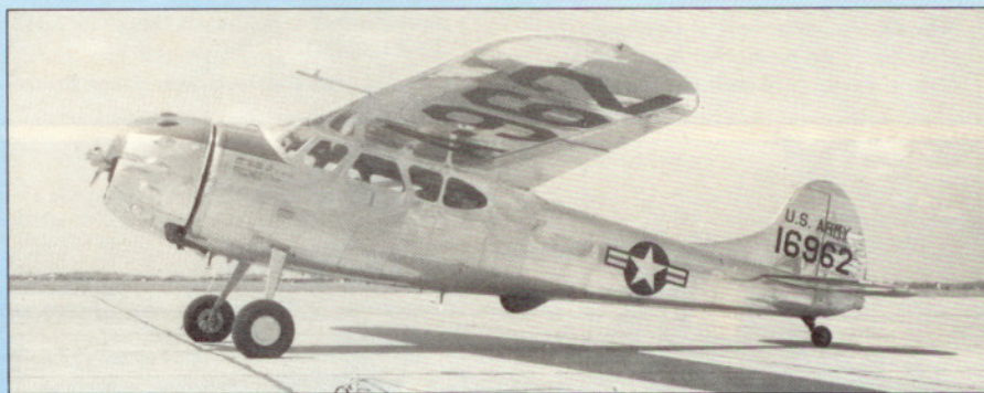
The LC-126C was the final military version of the Cessna 195 series. It had an extra-wide right door for loading litters and a window on the left side that could be opened as a camera port.
